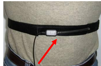
The rubber strap stretches when the abdomen expands during breathing.
